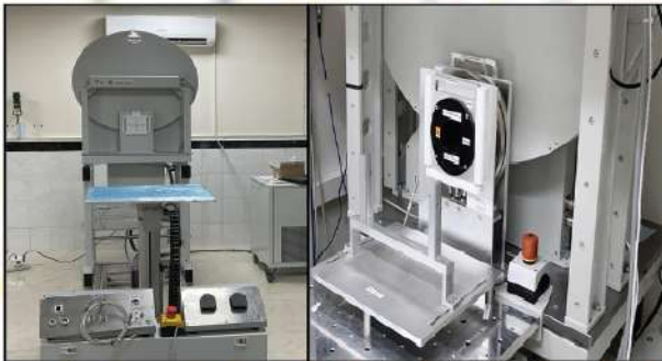
60kV X-ray Calibration System (PTW)
